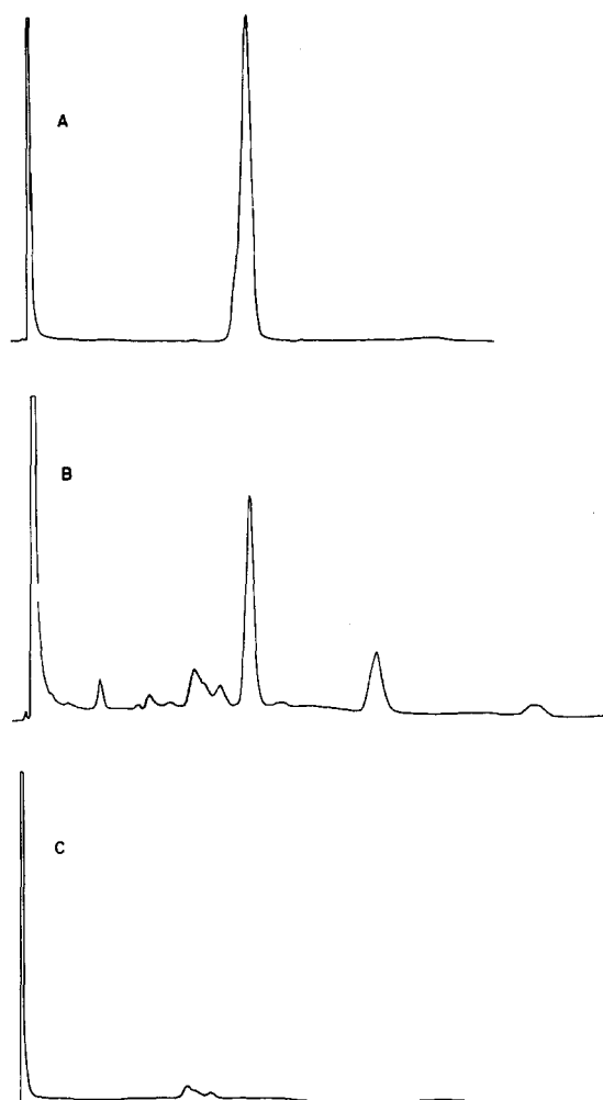
FIG. 2. Trilinolenin was methylated with 5.5-month-old boron trifluoride-methanol for 90 min at 120°C in a glass ampoule (A), a Teflon-lined screw-cap vial (B), or a vinyl-lined screw-cap vial (C). The destruction of the linolenic acid increased with decreasing inertness and tightness of the reaction vessel.
